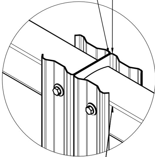
RAILS SCREWED INTO C-POSTS USING 2x 10gx16mm TEK SCREWS
